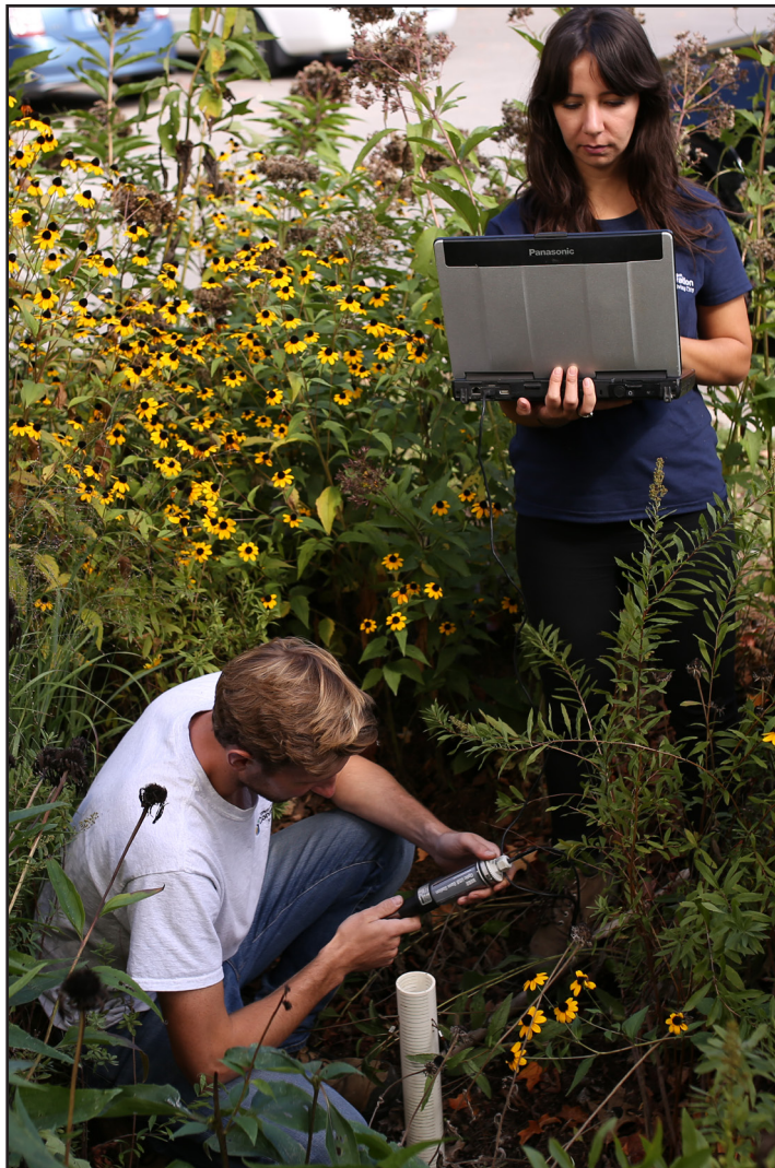
Figure 6. Continuous water level monitoring in a bioretention
